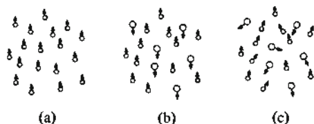
FIG. 5. Atomic magnetic moments in amorphous magnets: (a) ferromagnetic as in Fe 80 B 20 , (b) ferrimagnetic as in Gd 30 Co 70 , and (c) canted ferrimagnetic as in Tb 33 Fe 67 .
