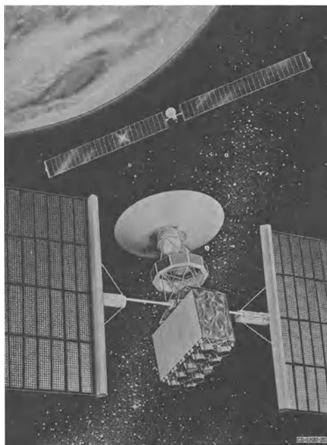
FIG. 4. Artist's representation of SEP (Solar Electric Propulsion System) Spacecraft. 25 KW power level.
