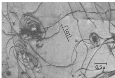
FIG. 3. A deformed copper alloy crystal containing hard particles. Electron micrograph showing interaction of dislocation lines with the second phase.
