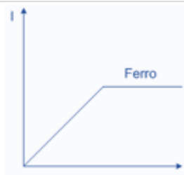
I-M curve for ferromagnetic materials
