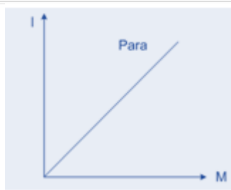
I-M curve for paramagnetic material
